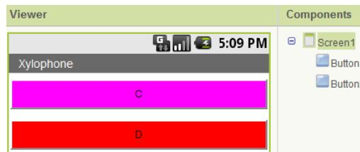
Figure 9-2. Placing buttons to create a keyboard
