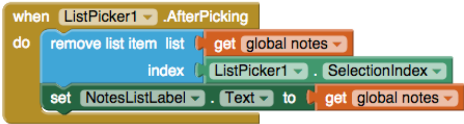
Figure 19-19. Removing an item by using ListPicker.SelectionIndex
