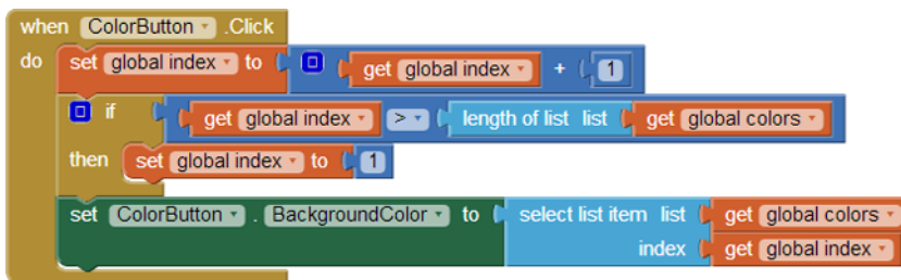
Figure 19-9. Using an if to check whether the index value is larger than the length of the list
