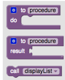
Figure 21-5. A call block appears in the Procedures drawer when you define a procedure
